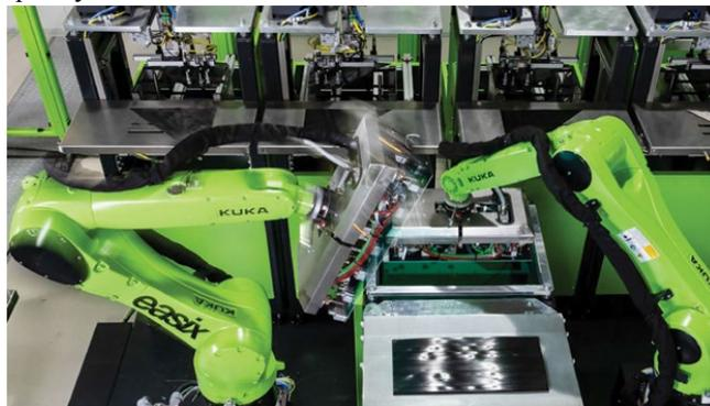
Figure 1. Tape stacking cell with high-speed articulated robots.
